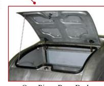
One-Piece Rear Body Upper Structure and Trunk Water Management System
